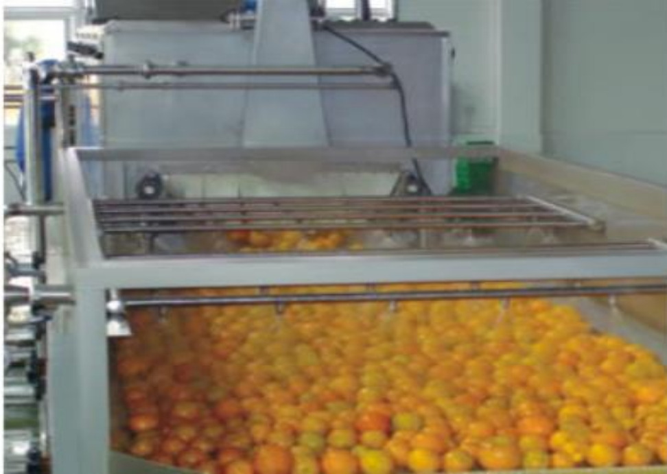
Figure 3.2. Roller with brush cleaning machine
